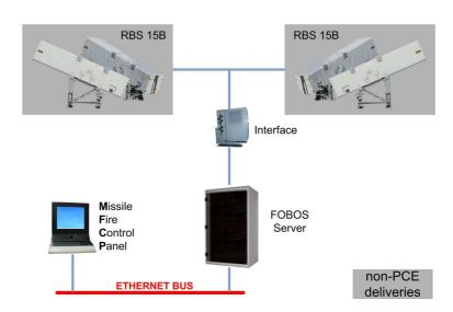
**FOBOS** can be used as a standalone system(on board) or in a connection with the **DEIMOS** fire control system, which enables extended functionality providing detailed graphical display of tactical situation, missile target data tables and missile flight trajectory. Missile fire control panel can be stand alone unit or it can be integrated within Tactical & Missile Console.
