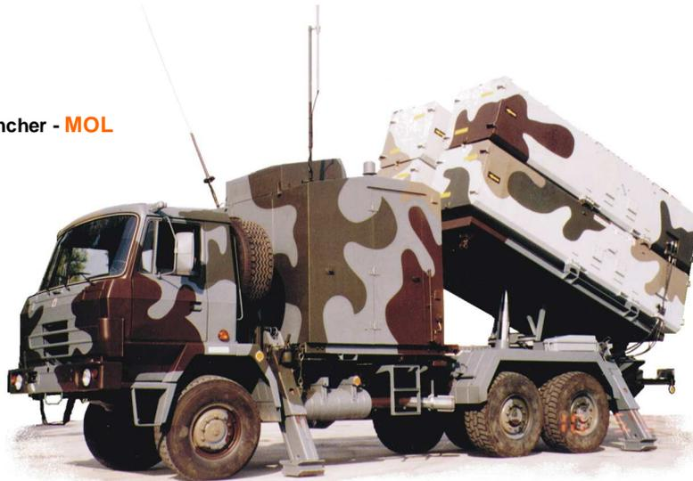
**FOBOS** is compact and fast missile launching control system, that was developed for Saab **RBS15B** missiles. It can control up to eight missiles, and can be installed on a ship or on a land vehicle.
